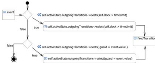
Fig. 6. Evaluation of guard conditions: StateMachineInstance#evalGuards
